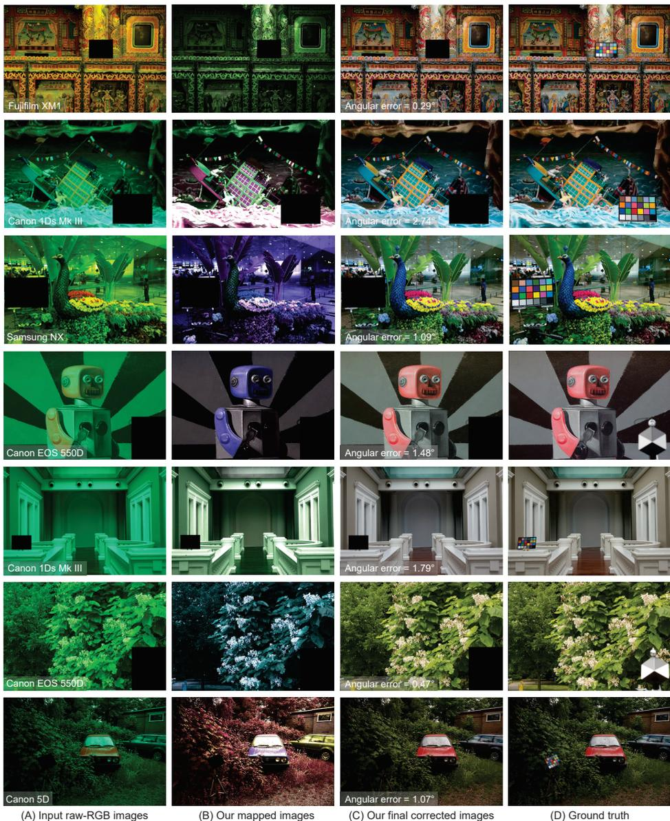
Figure 3: Additional qualitative results of our method. (A) Input raw-RGB images. (B) After mapping images in (A) to the learned space. (C) After correcting images in (A) based on our estimated illuminants. (D) Corrected by ground truth illuminants. Shown images are rendered in the sRGB color space by the camera imaging pipeline in [5] to aid visualization.
