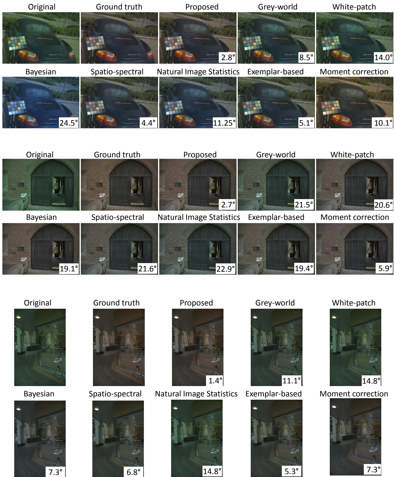
Figure 2: Corrected images using the estimated illuminant from two statistical methods and sox learning-based methods (including our proposed one). The angular error is given at the lower right corner of the image. The RAW images have been applied gamma function to boost the contrast for a better visualization. It is best viewed online.
