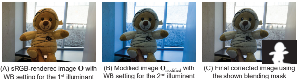
Figure 7. Our method can be used to correct or modify the WB settings for two-illuminant scenes. (A) Camera-rendered sRGB image with the WB settings used for the first illuminant. (B) Generated sRGB image for the second illuminant using our metadata. (C) Our final result after blending.
